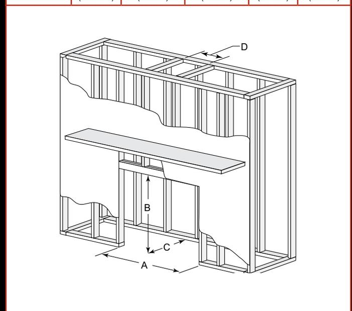
The rough framing dimensions shown represent the distance from stud to stud only and do not take into consideration the addition of drywall. Please refer to installation instructions for complete specifications and drawings when installing this product. Go to [heatilator.com](http://heatilator.com) to download.
