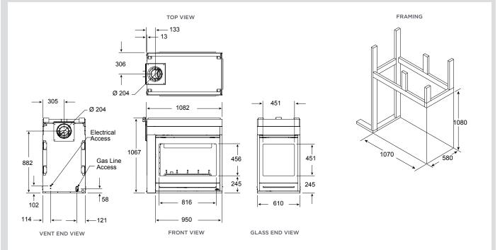
Dimensions above are in millimeters and for reference only. We recommend measuring individual units at installation. Assumes the use of 13mm gyprock. Refer to installation manual for detailed specifications on installing this product. Heat & Glo reserves the right to update units periodically. The flame and ember appearance may vary based on the type of fuel burned and the venting configuration used. Photos in this brochure may vary in color and dimension [size] from the actual product.
