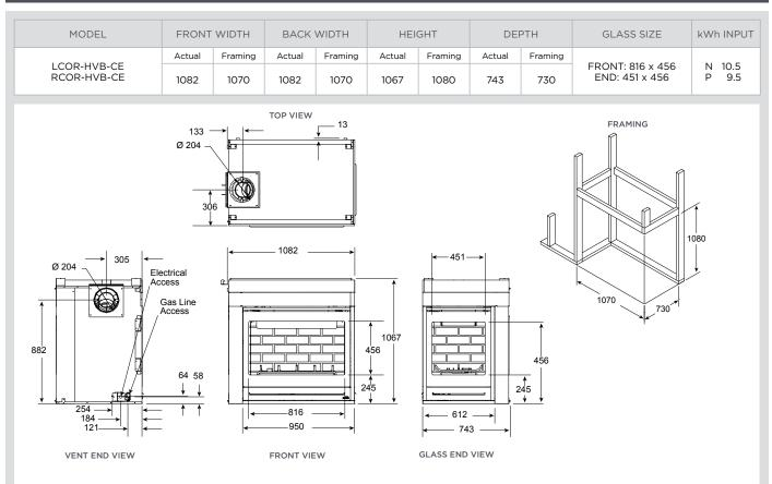
Dimensions above are in millimeters and for reference only. We recommend measuring individual units at installation. Assumes the use of 13mm gyprock. Refer to installation manual for detailed specifications on installing this product. Heat & Glo reserves the right to update units periodically. The flame and ember appearance may vary
