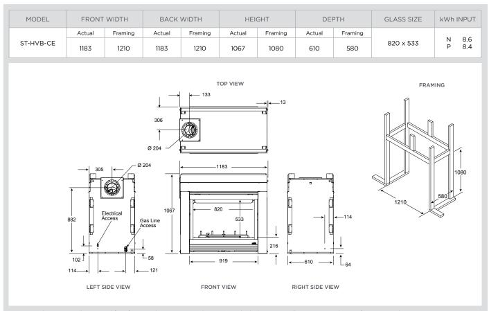
Dimensions above are in millimeters and for reference only. We recommend measuring individual units at installation. Assumes the use of 13mm gyprock. Refer to installation manual for detailed specifications on installing this product. Heat & Glo reserves the right to update units periodically. The flame and ember appearance may vary based on the type of fuel burned and the venting configuration used. Photos in this brochure may vary in color and dimension [size] from the actual product.
