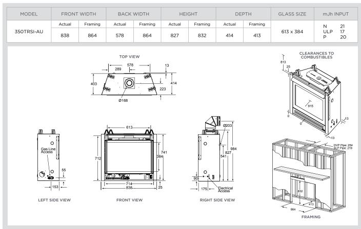
Dimensions above are in millimeters and for reference only. We recommend measuring individual units at installation. Assumes the use of 10 mm gyprock. Refer to installation manual for detailed specifications on installing this product. Heat & Glo reserves the right to update units periodically. The flame and ember appearance may vary based on the type of fuel burned and the venting configuration used. Photos in this brochure may vary in color and dimension [size] from the actual product.
