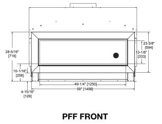
The PFF decorative front has an installed depth of 3/4" [19mm], measured from the front of the non-combustible finishing material to the front of the decorative front.
