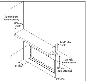
**Back Wall Clearance** – The appliance may be placed against a combustible back wall.
